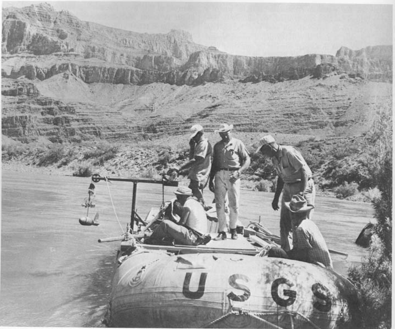
FIGURE 86.—Flow-measurement gear being readied for observations of velocity and depth. The 100-pound weight hangs below the current meter from a cable on the winch.
