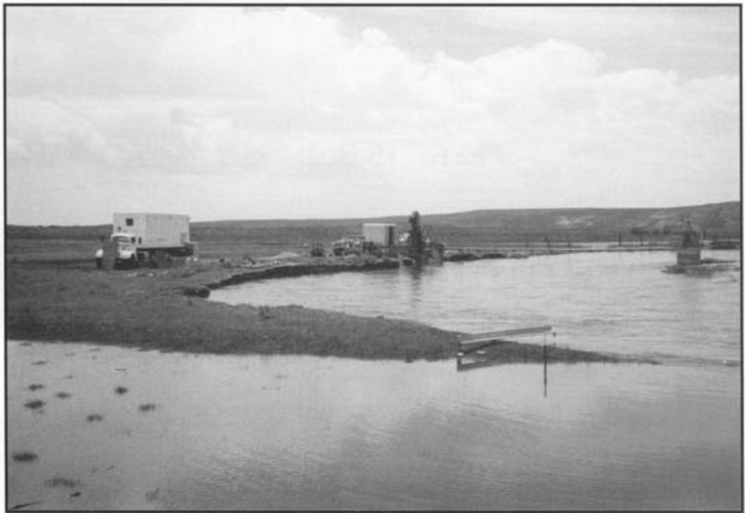
Figure 15. Site of the bedload trap at low flow and high flow. A , Looking downstream at low flow, showing the low gravel bar left of center of the channel and just upstream from the trap. At far left can be seen the levee built to prevent the water from flowing into the diversion channel, the spoil from which rises above the flat lower surface. B , Looking upstream at a stage at which high flow inundates the flood plain.
