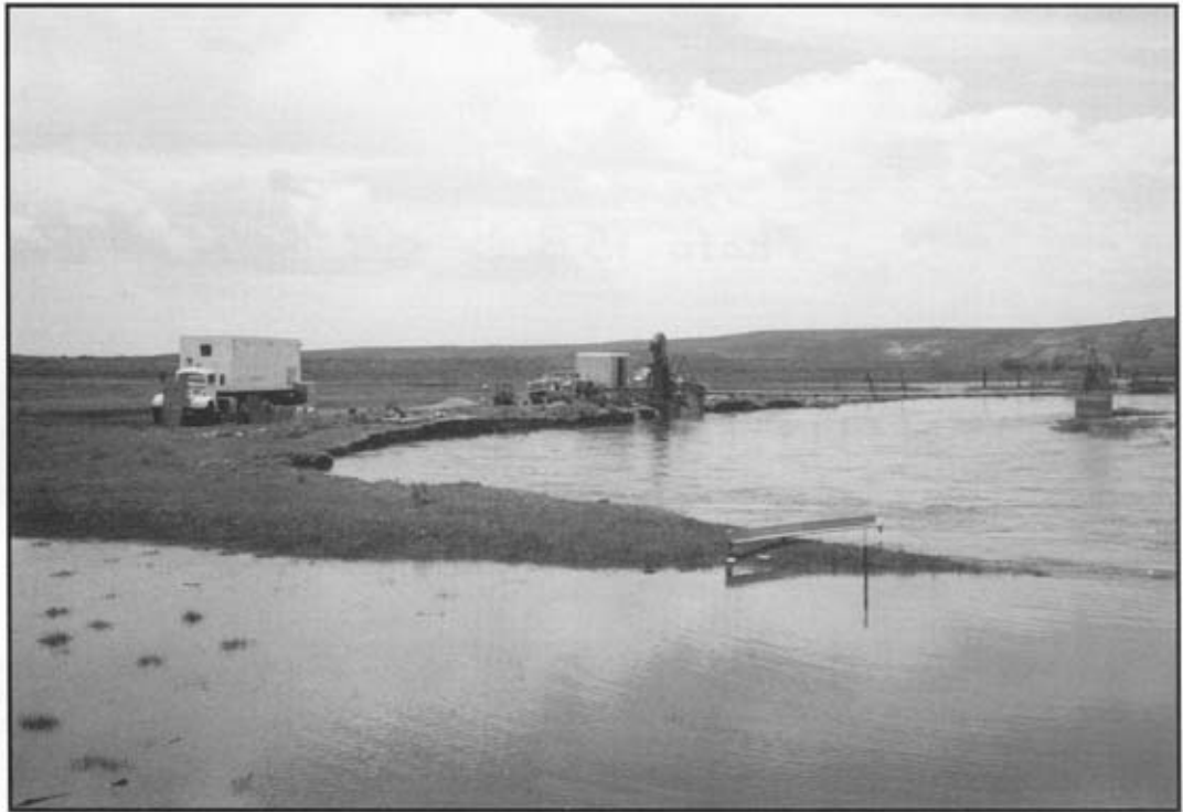
Figure 15. Site of the bedload trap at low flow and high flow. A , Looking downstream at low flow, showing the low gravel bar left of center of the channel and just upstream from the trap. At far left can be seen the levee built to prevent the water from flowing into the diversion channel, the spoil from which rises above the flat lower surface. B , Looking upstream at a stage at which high flow inundates the flood plain.
