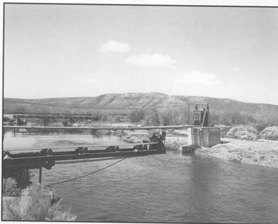
Figure 22. The bedload trap on East Fork River (continued). F , The endless belts leading first downstream from the weighing hopper, and the orthogonal belt extending over the river for returning bedload to the channel. G , View from right bank looking upstream; the endless belt in the foreground carries sediment back to the river after it is weighed and sampled.
