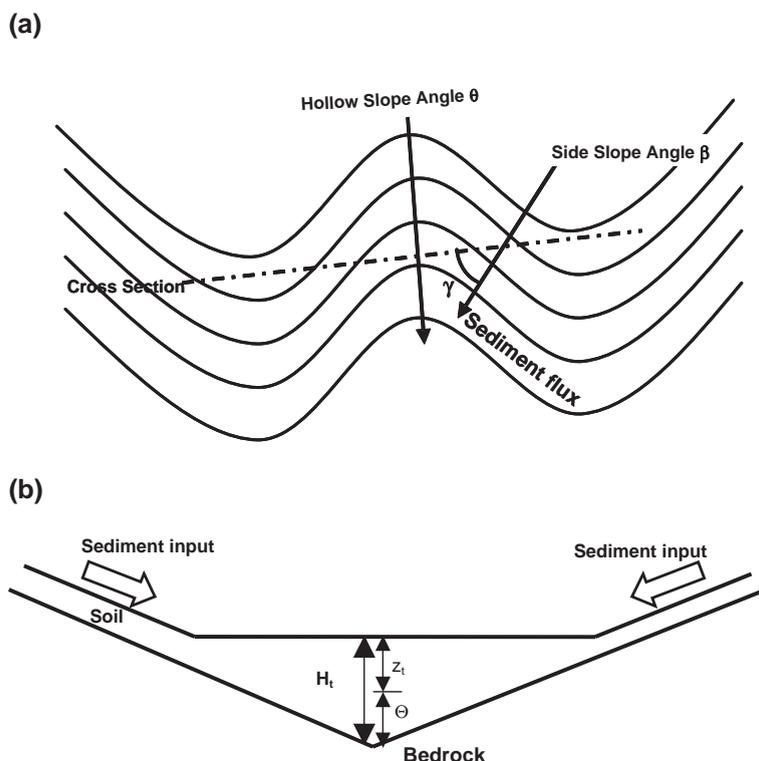
Fig. 2. The geometry of hollows at Tennessee Valley: (a) plan view and (b) simplified cross sectional view used for modeling soil thickness during sediment infilling. Symbols:  $\beta$  is side slope angle,  $\theta$  is hollow slope angle,  $H$  is soil thickness,  $z$  is depth from ground surface to soil layer of interest, and  $\Theta$  is the distance from the soil layer of interest to bedrock.
