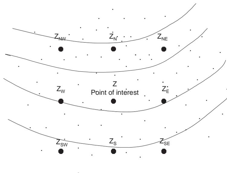
Fig. 4. An illustration of how grid points were used to calculate topographic attributes (Heimsath et al., 1997). Actual cm-accuracy survey points (small dots) were used, using a Kriging method, to generate grid points (filled dots). Contour lines were generated using *Surfer*® software from the grid point data.  $Z$  is the elevation in meters relative to local reference point.
