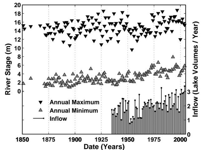
Figure 9. Yearly maximum and minimum river stages and lake inflow. River stages measured at Red River Landing 8 km upstream of the tie channel. Inflow represents the number of times the oxbow lake fills over the course of the year and is derived from daily stage data. The stage data show a progressive rise in both the minimum and maximum elevations over time. The average yearly inflow is two lake volumes but also shows a slight increase over time.
