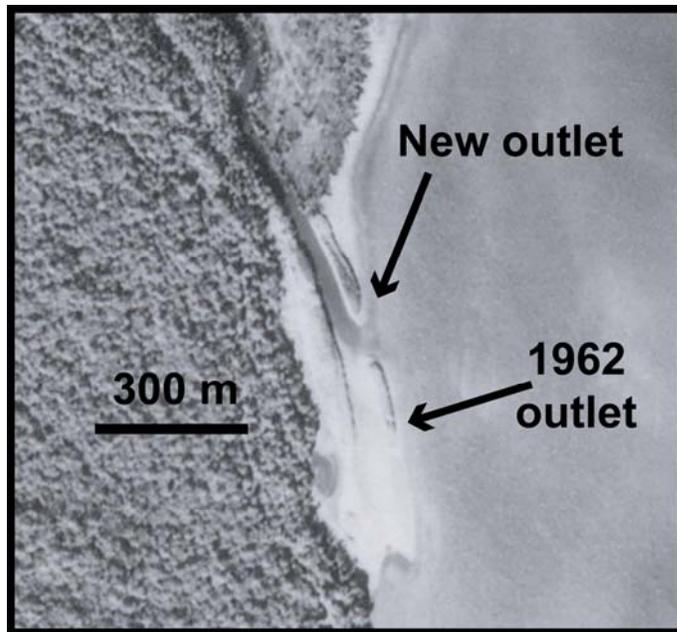
Figure 7. 1983 aerial photograph of channel outlet showing breach in left channel levee that became the present day channel course. The maximum extent of the channel in 1962 is shown with the arrow. Note the minimal advancement of the channel lakeward since 1962. This hiatus of channel advancement appears to be in response to the increase in channel base level due to dam construction in 1965.
