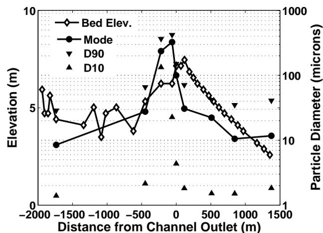
Figure 6. Bathymetric survey from the channel into the lake and grain size characteristics of bed samples collected along the survey. The 0 location on the distance axis marks the end of the exposed channel levees. The prominent rise in the bed at the channel outlet marks the mouth bar which lies between the channel levees at the outlet. The slope of the channel bed is 0.0008, and the slope on the delta front (the last 1000 m) is 0.0034.
