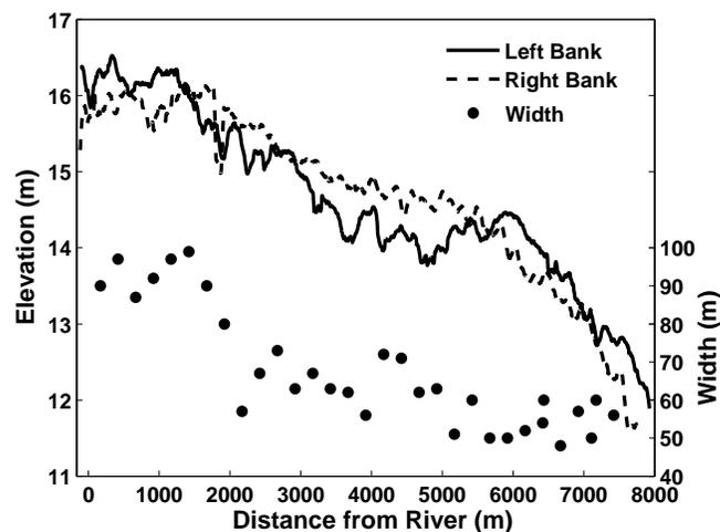
Figure 3. Long profile of tie channel levee crest elevations and channel widths measured between crests. Data from 2003 ALSM survey of site. Elevation data smoothed by averaging over a 100 m window. Width measurements made approximately every 250 m along the channel. Source of data: Concepts, Watershed 2005.
