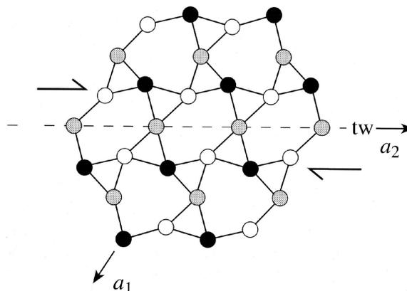
Figure 1. Model for structure of Dauphiné twin (tw) in quartz produced by shear. Only silicon atoms are shown (circles); gray shades indicate different levels along *c*-axis; *a*<sub>1</sub> and *a*<sub>2</sub> are crystallographic axes.
