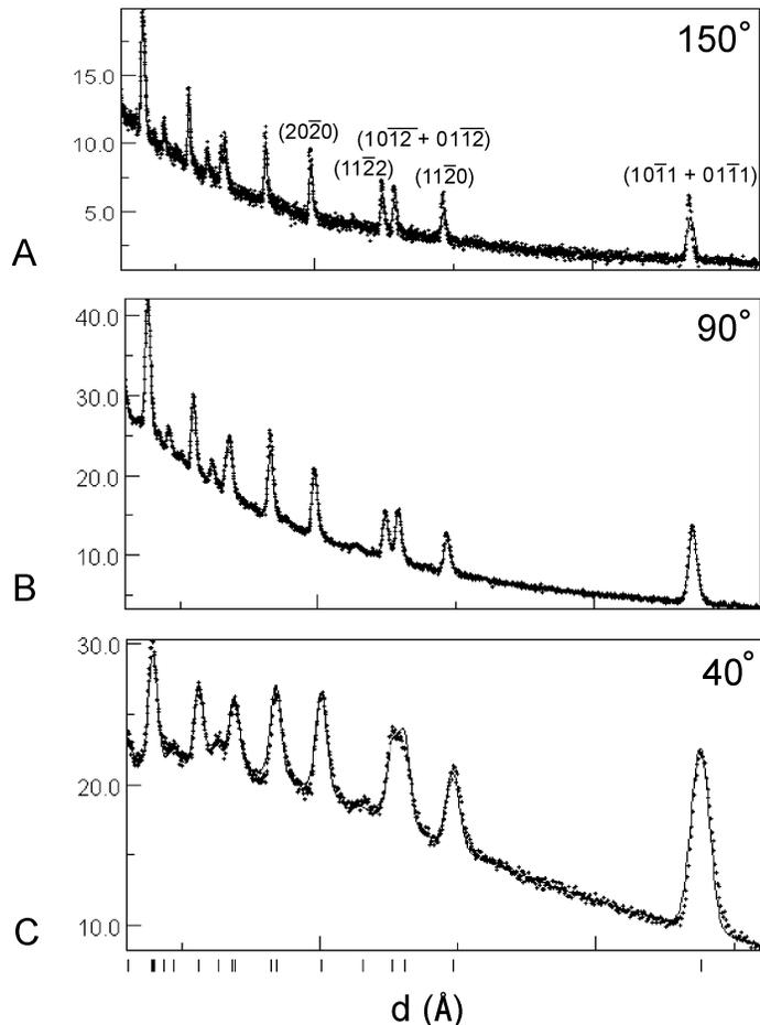
**Figure 3.** Time-of-flight neutron diffraction spectra for Vredefort quartzite that were used for Rietveld texture refinement. Examples of  $150^\circ$  (A),  $90^\circ$  (B), and  $40^\circ$  (C) detectors. Dot pattern is measured spectrum, and line indicates Rietveld fit. Some quartz diffraction peaks are indexed, with calculated peak positions indicated below. Abscissa is *d*-spacing.
