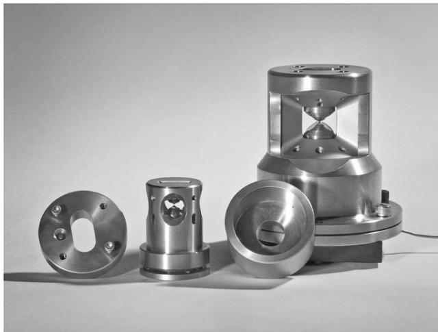
FIG. 3. Picture of the loading frame and two rDACs. From left to right: top spacer for Merkel style panoramic rDAC, Merkel style panoramic rDAC, bottom spacer, and Mao-type panoramic rDAC, and gas membrane inside assembled loading frame.
