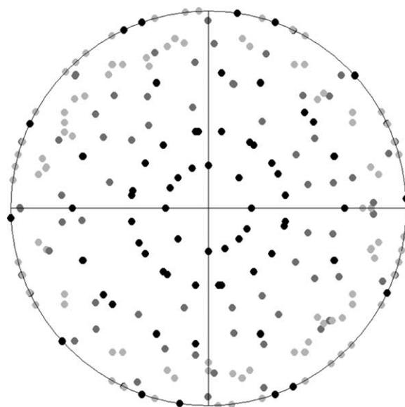
Fig. 4. Pole figure coverage. Sample was rotated about the cylinder axis (which was vertical) to 0, 45, 90, 135, 202.5, and 242°. Thirty detector panels on three rings at different Bragg angles were used. 140° ring, light gray; 90° ring; gray, 40° ring; black.
