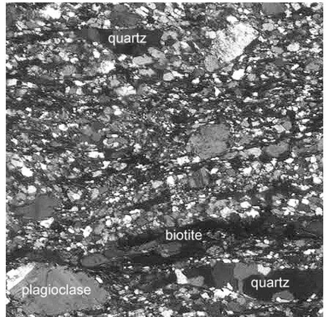
Fig. 2. Photomicrograph of PC 418, crossed polars. Width is 4 mm. Section is normal to the foliation plane and contains the lineation.
