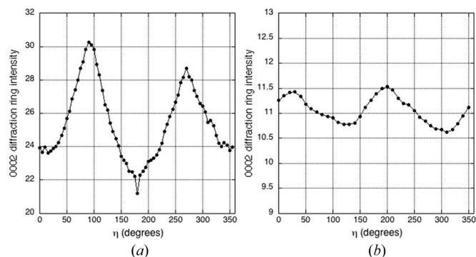
**Figure 4** (0002) Debye ring intensity variation (in arbitrary units) of (a) dinosaur tendon and (b) salmon scale. The dinosaur sample clearly shows a stronger texture than the salmon scale, confirmed in the analysis by the texture results.
