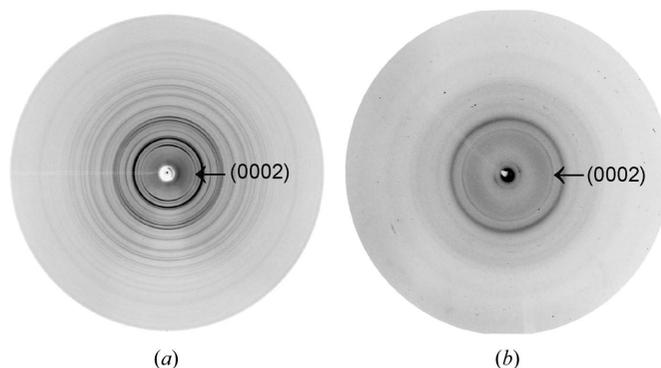
**Figure 1** Two-dimensional synchrotron diffraction images as they were used in the Rietveld analysis. (*a*) Dinosaur tendon recorded using an image plate. (*b*) Salmon scale recorded using a CCD camera. The (0002) Debye rings show strong intensity variation for dinosaur and a lesser one for salmon scale. These variations are indicative of texture.
