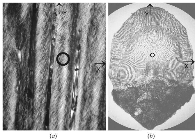
**Figure 2** Photomicrograph of (a) a thin section of dinosaur tendon (UCMP 128383) showing well organized longitudinal Haversian canals, and (b) Atlantic salmon scale. Image dimensions are 1 mm across for the dinosaur tendon, and 4 mm for the salmon scale. The sample coordinate system (*XYZ*) used in this study is indicated. The circle indicates the location of the texture analysis.
