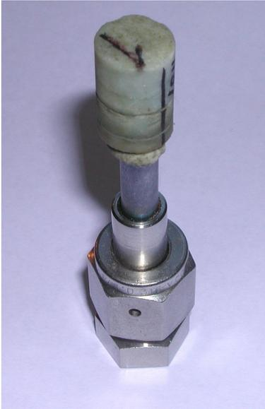
Figure 1. Cylinder of rock, marked with an arrow to indicate orientation, mounted on a sample holder.
