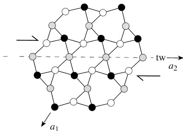
**Fig. 1** Model for the structure of a mechanical Dauphiné twin produced by shear, [0001] projection (Schubnikov and Zinslerling 1932). Twin plane ( $tw$ ) and sense of shear are indicated. Only Si atoms are shown with gray shades different  $z$ -coordinates
