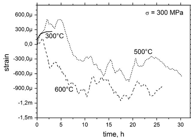
**Fig. 3** Plot of microstrain as function of time for samples N2-1 (300°C), N2-9 (500°C), N2-11 (600°C)
