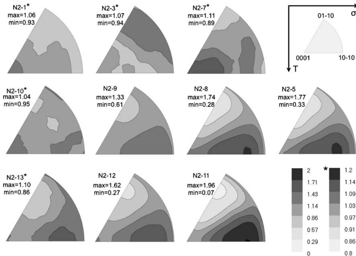
**Fig. 8** Inverse pole figures documenting variation of texture with temperature and differential stress. *Top row* is 300°C, *center row* 500°C and *bottom row* 600°C. For stresses see Table 1. Axial
