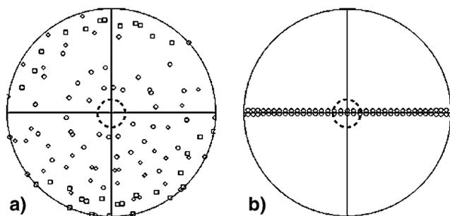
**Fig. 4** Pole figure coverage **a** with HIPPO neutron diffraction data (circles are 150° detectors, squares 90° and diamonds 40°) and **b** with a single synchrotron X-ray diffraction image. Compression direction is in the center (dashed ring)
