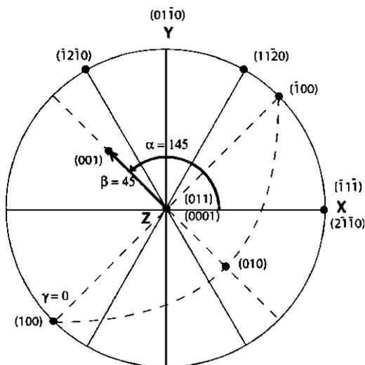
Fig. 5. Definition of coordinate system and of Euler angles  $\alpha$ ,  $\beta$  and  $\gamma$  for hcp and bcc crystals. The hcp crystal is in the standard orthogonal coordinate system  $X, Y, Z$ . For bcc the orientation variant 1  $\{\alpha' = 145^\circ, \beta' = 45^\circ, \gamma' = 0^\circ\}$  is shown relative to the hcp crystal.
