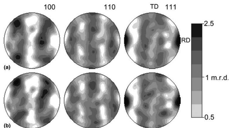
Fig. 3. Experimental pole figures of cubic Zr obtained measured in situ at 950 °C with TOF neutron diffraction. (a) First heating cycle, (b) second heating cycle. Equal area projection, rolling direction (RD) and transverse direction (TD) are indicated.
