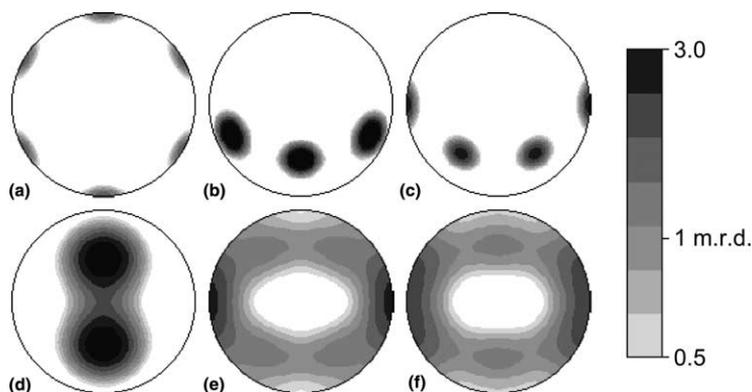
Fig. 4. Ideal components of the hcp texture. (a)  $11\bar{2}0$  pole figure for component  $g_1$ , (b)  $11\bar{2}0$  pole figure for  $g_2$ , (c)  $11\bar{2}0$  pole figure for  $g_3$ , (d)  $0001$  pole figure with all three components added for volume fractions defined in Table 2, (e)  $10\bar{1}0$  pole figure, (f)  $11\bar{2}0$  pole figure. Equal area projection.
