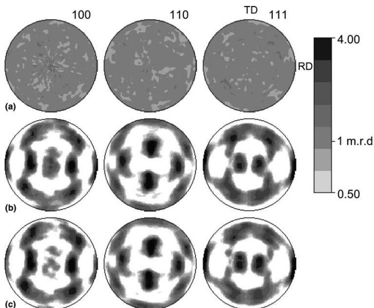
Fig. 7. Simulated bcc pole figures obtained from the hcp texture in Fig. 3(b), based on Burgers relation. (a) Transformation texture applied to all orientations with all six symmetry variants. (b) Transformation applied to orientations near  $g_3$ , without variant selection. (c) Transformation applied to orientations near  $g_3$ , with variant selection as described in the text. Equal area projection.
