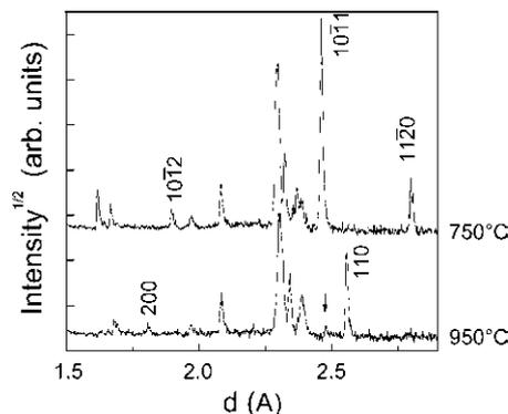
Fig. 1. Neutron diffraction patterns obtained from rolled zirconium at 750 °C (hcp phase) and 950 °C (bcc phase). Diffraction peaks without  $hkl$  indices are dominated by beam interaction with the high-temperature Nb furnace. Indexed diffraction peaks have been used for the texture analysis. The arrow indicates a small residual fraction of hcp Zr in the bcc-transformed sample.
