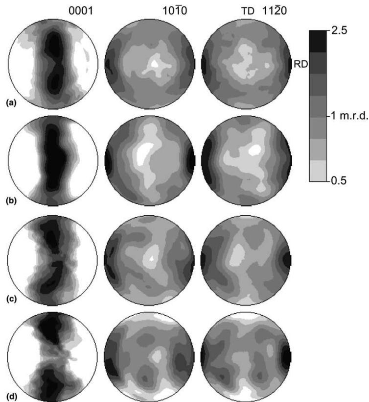
Fig. 2. Experimental pole figures of hexagonal Zr obtained during thermal cycling (cf. Table 1). (a) Room temperature, (b) 750 °C (before phase transformation), (c) 750 °C (after phase transformation), (d) 750 °C (after second phase transformation). Equal area projection, rolling direction (RD) and transverse direction (TD) are indicated. (a) Measured with an X-ray pole figure goniometer, (b)–(d) with TOF neutron diffraction.
