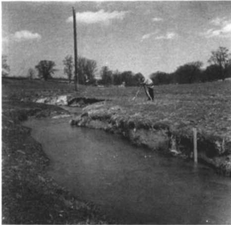
Figure 3. Watts Branch in May 1953, looking upstream toward area where cross sections were established. Staff gage at natural section in right foreground and where bankfull stage was determined.
