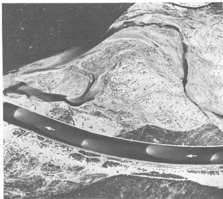
Fig. 13.1. Aerial photograph of the Colorado River near Needles, California. Controlled discharge and bank stabilization led to an unusual symmetry of moving bars on the bed. The direction of water flow is shown by arrows
